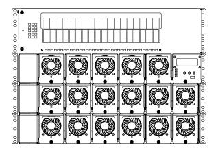
Description: -48VDC power system @ up to 555 Amperes, 25000 Watts max.
